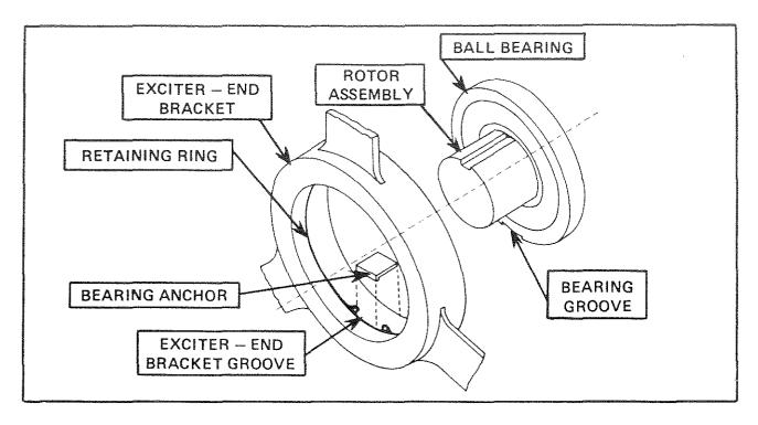
EXCITER - END BRACKET, BEARING AND BEARING ANCHOR ASSEMBLY
