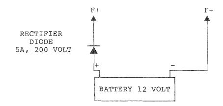
To flash the field while spinning at 1800 RPM, diode must be in + lead of battery as shown here.
