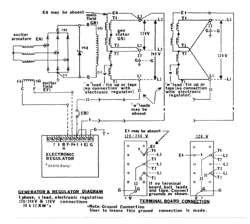
GENERATOR & REGULATOR DIAGRAM 1-PHASE, 4-LEAD, ELECTRONIC REGULATION 120/240 V & 120 CONNECTIONS
