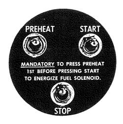
Should the engine not start when Start Switch is depressed for 10 to 12 seconds, wait 30 seconds and repeat Step 3 with adequate preheat time. Never run the starter motor for more than 30 seconds at a time.
