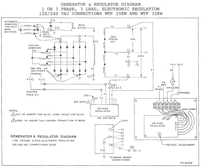
Note: Never connect terminal E1 to terminal 4. Loss of sensing voltage and maximum generator voltage would result.
